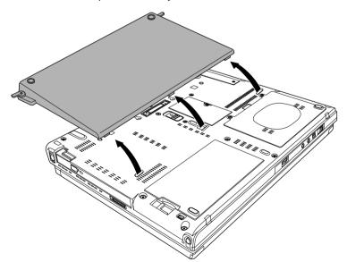
Figure 6-7 Removing the Slice Expansion Battery
